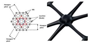
The Tensar InterAx geogrid uses the distinct stabilisation function as defined in ISO 10318 to minimise the movements of unbound granular material in road, rail and other trafficked areas. Extensive performance testing has demonstrated that when included as a component of a mechanically stabilised layer, the mechanical behaviour of the unbound layer is improved. The characteristics below allow product identification only.
